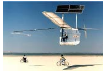
Gossamer Penguin (1980) 1 st manned solar powered flight
