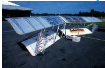
Solar Riser (1979) manned, battery solar charged for short flights
