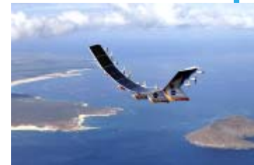
Helios (1999) unmanned, flew at > 29'000 m
